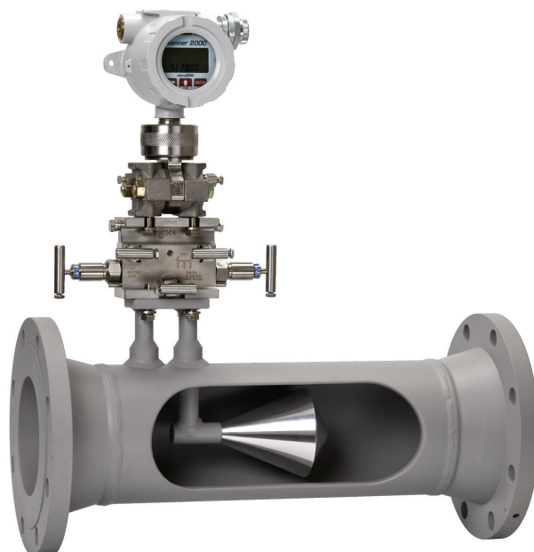
NUFLO DP cone meter technology with Scanner* flow computer, which computes volume, mass, and energy amounts for many types of fluid flow.
